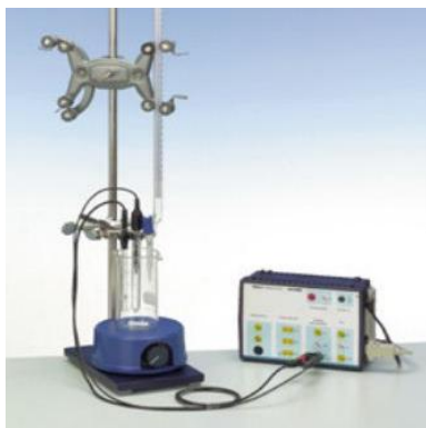
Figure B2. Left: A titration set up with a \text{H}^+ ion-selective electrode (also called a pH meter), and the equation by which measured [\text{H}^+] is converted to pH. Right: Example titration data measured using a pH meter, where red dots are individual measurements, and the yellow line is the equivalence point.
